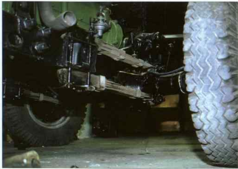
Left upper photos show detail of front left wheel plus steering handle. Other photos show details of right wheel with longitudinal quarter elliptical springs. Note also exhaust pipe.
