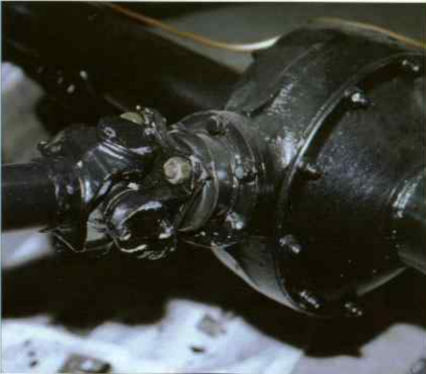
Photos on both pages show rear vehicle frame and transmission with torque transition on rear wheels. Well seen is differential with cardan shaft and longitudinal half elliptical springs with shock absorbers. Note also high pressure pipes for brake fluid distribution to hydraulic brakes.
