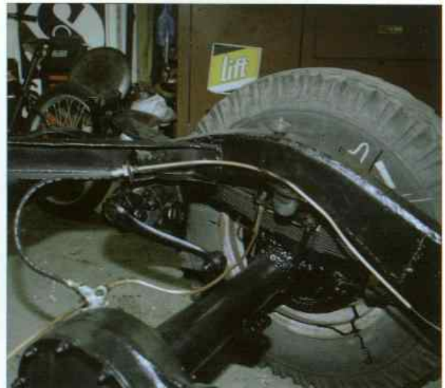
Photos on both pages show rear vehicle frame and transmission with torque transition on rear wheels. Well seen is differential with cardan shaft and longitudinal half elliptical springs with shock absorbers. Note also high pressure pipes for brake fluid distribution to hydraulic brakes.
