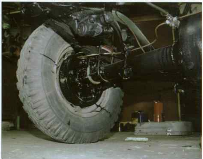
Photos on both pages show rear vehicle frame and transmission with torque transition on rear wheels. Well seen is differential with cardan shaft and longitudinal half elliptical springs with shock absorbers. Note also high pressure pipes for brake fluid distribution to hydraulic brakes.
