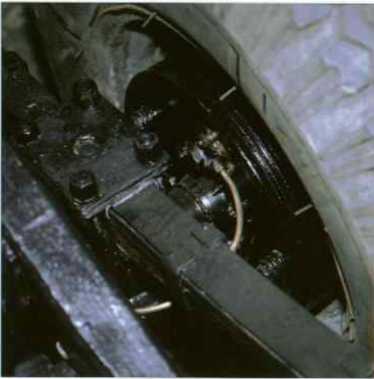
Photos on both pages show rear vehicle frame and transmission with torque transition on rear wheels. Well seen is differential with cardan shaft and longitudinal half elliptical springs with shock absorbers. Note also high pressure pipes for brake fluid distribution to hydraulic brakes.
