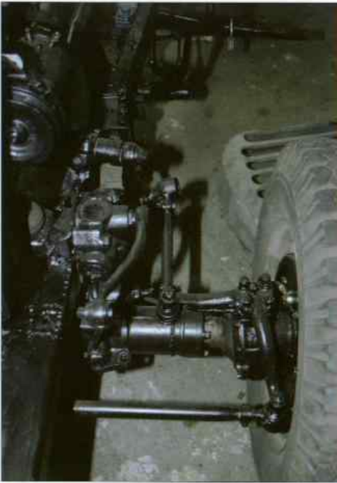
Left upper photos show detail of front left wheel plus steering handle. Other photos show details of right wheel with longitudinal quarter elliptical springs. Note also exhaust pipe.
