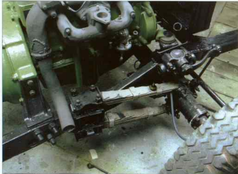
Left upper photos show detail of front left wheel plus steering handle. Other photos show details of right wheel with longitudinal quarter elliptical springs. Note also exhaust pipe.
